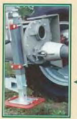
Hose full systems feature double inlets, internal check values, and quick coupler connections on both ends of the power tower. Water pick-up optional on last tower.
