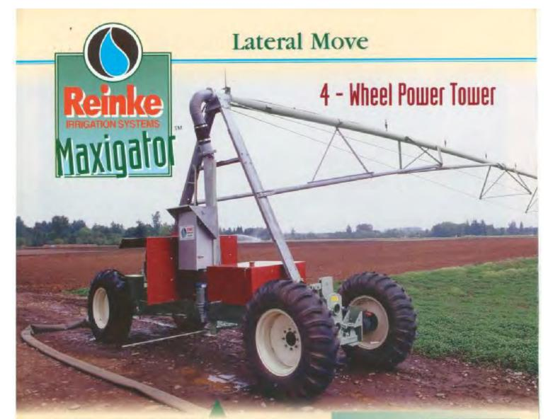
Get maximum pulling power on large fields with the Reinke 4-wheel drive power tower. This unit matches the demands of higher water flow requirements of large boses by providing reliable positive traction and labor savings.
